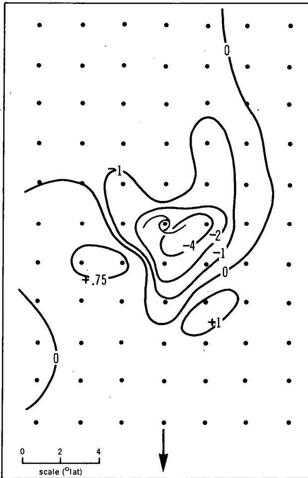
Fig 5 Pattern of low-level divergence around a tropical cyclone in the southern hemisphere with respect to its direction of motion shown by the arrow. This pattern was obtained after inverting the revised divergence field of Fig 4 and rotating it through 90^\circ
