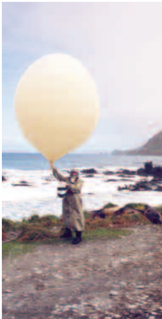
Fig. 1 Launch of an ozone sonde at Macquarie Island (photo by Jim Easson, Observations and Engineering Branch, Bureau of Meteorology).
