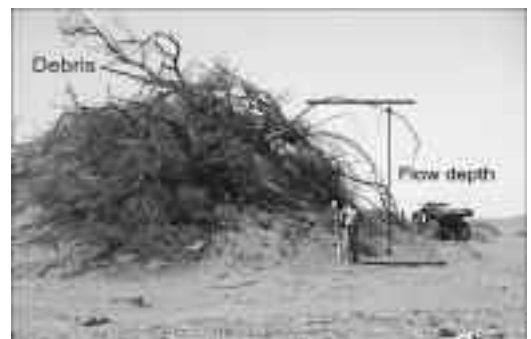
Fig. 5 Remnant of dune near Tubridgi Point with debris in tree on crest of dune. Note depth of marine inundation. Dune is located at the rear of the beach, so the actual depth of marine inundation here is several metres greater than the height of debris above immediate ground level.
