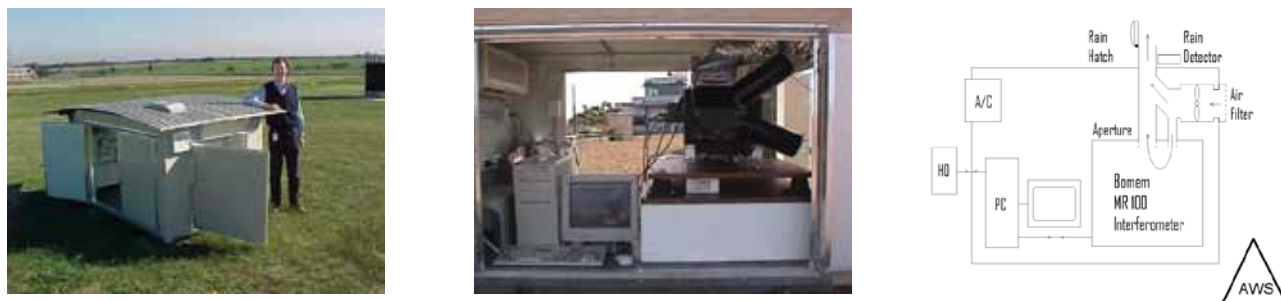
Fig. 1 The enclosure at Melbourne Airport (left), the layout of the interferometer and computer in the enclosure (centre) and a schematic diagram of the B-AERI (right) including an automatic weather station (AWS).
