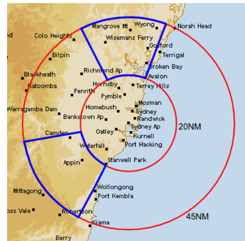
Figure 2: 20NM and 45NM range rings (red) around Sydney Airport with 330-020° and 210-260° sectors (blue) indicated.
