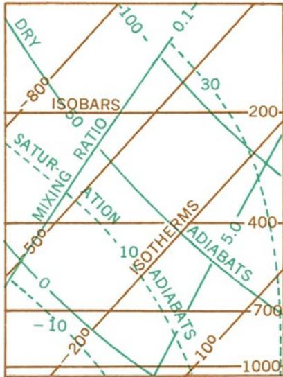
The aerological diagram is used by forecasters to view the current vertical distribution of temperature and moisture in the troposphere, and to determine the atmosphere's stability.
