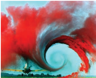
Wake Vortex Study at Wallops Island. The air flow from the wing of this agricultural plane is made visible by a technique that uses colored smoke rising from the ground. Image courtesy of NASA, traces the aircraft's wake vortex, which exerts a powerful influence on the flow field behind the plane.
