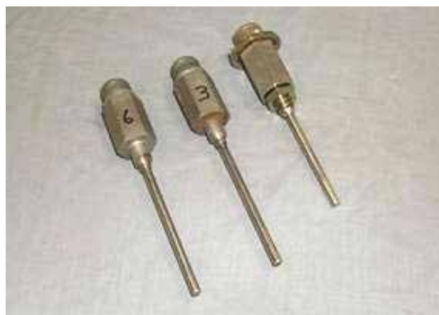
Figure 6. Three versions of the platinum-resistance sensors used in Bureau AWS since the 1980s.
