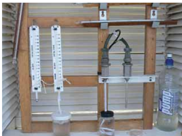
Figure 5. The internal view of a small Stevenson screen set up with both in-glass and platinum resistance probes. Maximum and minimum thermometers are in the upper right, and a spare terrestrial minimum thermometer is in the top left. The photo was taken during the site audit by the Regional Instrument Centre of the Hobart Airport site in 2010.
