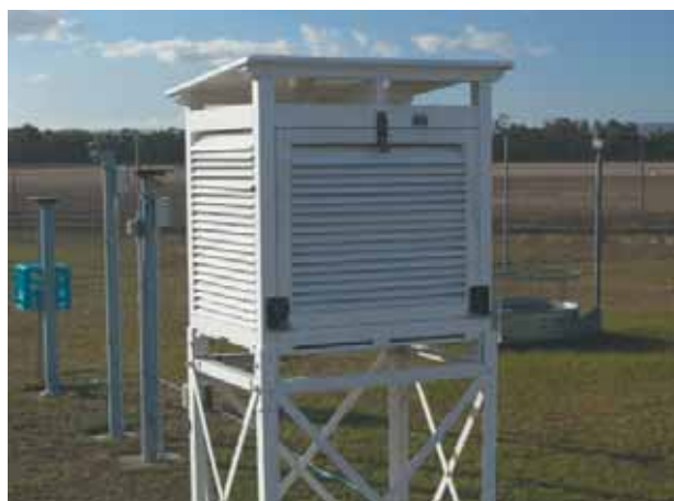
Figure 4. Small Stevenson screen used at the majority of SAT observing sites.
