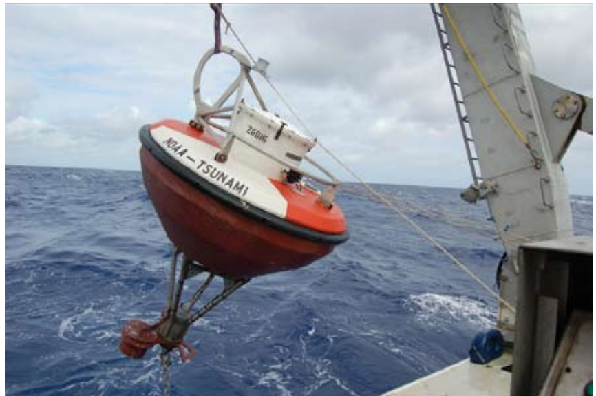
Deep Ocean Tsunami Detection Buoys will form part of the Bureau’s enhanced sea-level monitoring network.
