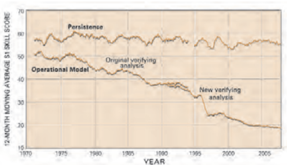
Figure 29. Values for the S1 skill score, a measure of the errors in prediction (lower score indicates higher skill), for 24-hour forecasts of mean sea-level pressure from operational and persistence prognoses over the Australian region. The values shown are 12-month running means. The persistence predictions, based on the assumption that today's pattern will continue unchanged tomorrow, show relatively large errors and no long-term trend. The original base analysis used for verification purposes has been discontinued. The results during the overlap period show a slight shift in the measure of skill, but the trends are similar.
