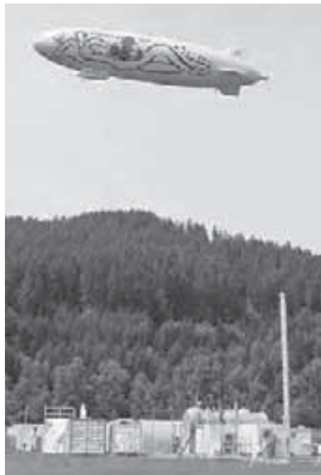
The Zeppelin NT circles around the ARM Mobile Facility in Heselbach, Germany, collecting air samples and recording vertical air column data. Deployment was part of the Convective and Orographically-induced Precipitation Study, conducted by the World Meteorological Organization's World Weather Research Programme in the latter half of 2007.
