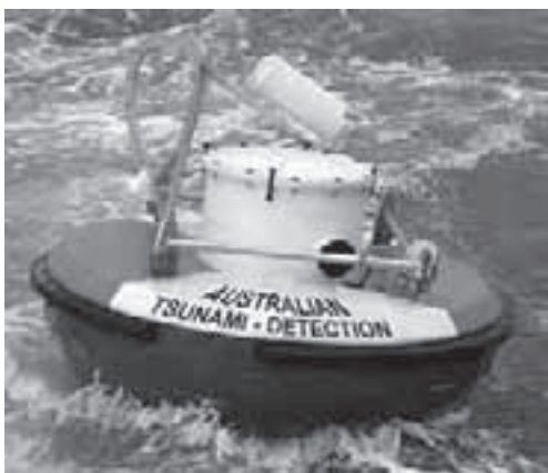
A deep ocean tsunami detection buoy shortly after its deployment in the Coral Sea.
