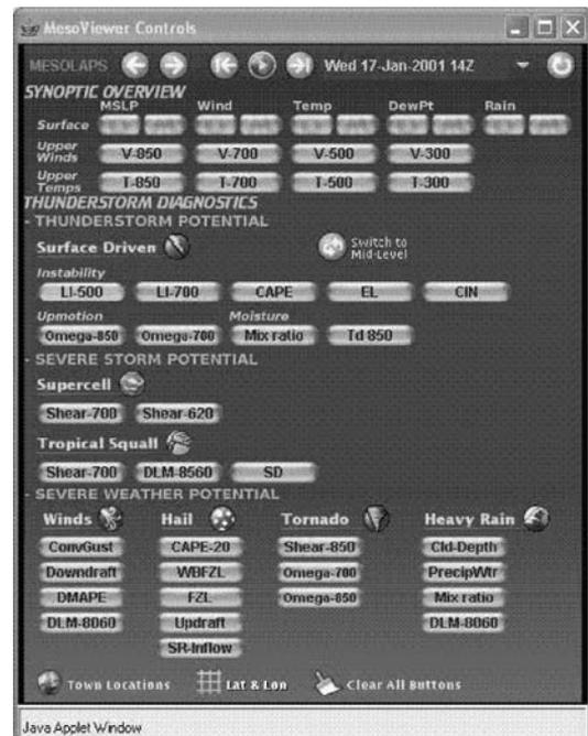
fields are based on thunderstorm conceptual models relating up-motion, moisture, instability and shear to thunderstorm initiation, development and structure. One of the key elements of the system is a web-based graphical user interface (GUI) referred to as the mesoviewer (Fig. 1). Forecasters can view three-hourly MesoLAPS NWP data (Puri et al. 1998) in a way that reinforces the (severe) thunderstorm forecast process.
