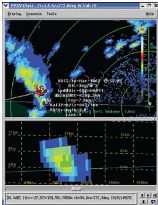
**Fig. 13** 3D-Rapic display from Marburg radar at 1652 UTC (0252 LST). (a) PPI and simulated RHI display (along light blue line through cell 1062 in PPI) with WDSS overlay. WDSS tracks as described in Fig. 11(a). (b) PPI display with TITAN overlay. Past 10-minute TITAN positions in light blue, TITAN 10-minute forecast positions out to 60 minutes in purple.
