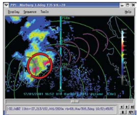
warning products, guaranteeing consistency. For example, in Fig. 14(a) with the forecaster having decided on the validity of the TITAN forecast track (the option exists to interactively change the forecast track) and adding the warning area, Fig. 14(b) (a site-specific
