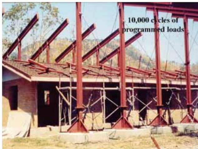
Fig. 5 Full size houses that exhibited premature failure.
