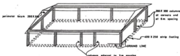
in the engineered cottage construction would have only a local effect, and would not lead to the collapse of the total house as frequently occurred to houses struck by cyclone Tracy.
