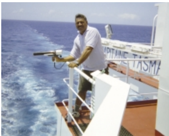
Crew on a Pacific islands trader contribute to monitoring ocean conditions, here using instruments that record data in the upper one kilometre of the ocean.
