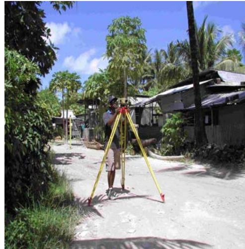
Mr Andrick Lal conducting a precise differential levelling survey in Betio, Tarawa, Kiribati.
