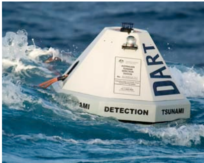
Deep-ocean tsunami detection buoy.
