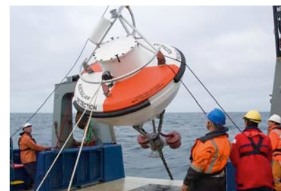
The deployment of a DART™ buoy in the Tasman Sea.
