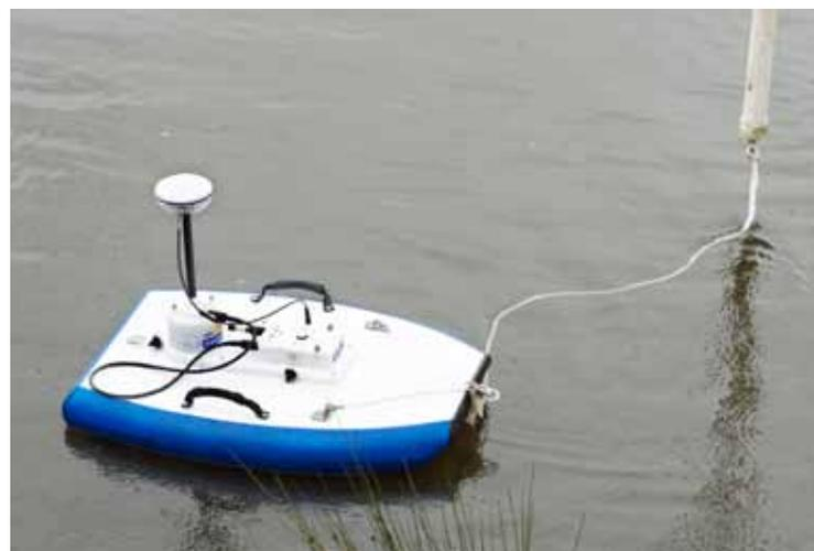
Sontech M9 acoustic doppler current profiler on a travellerway.
