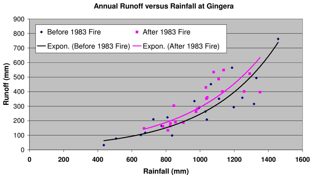
Figure 5 Curves of rainfall and runoff pre 1983 and post 1983 bushfire.
