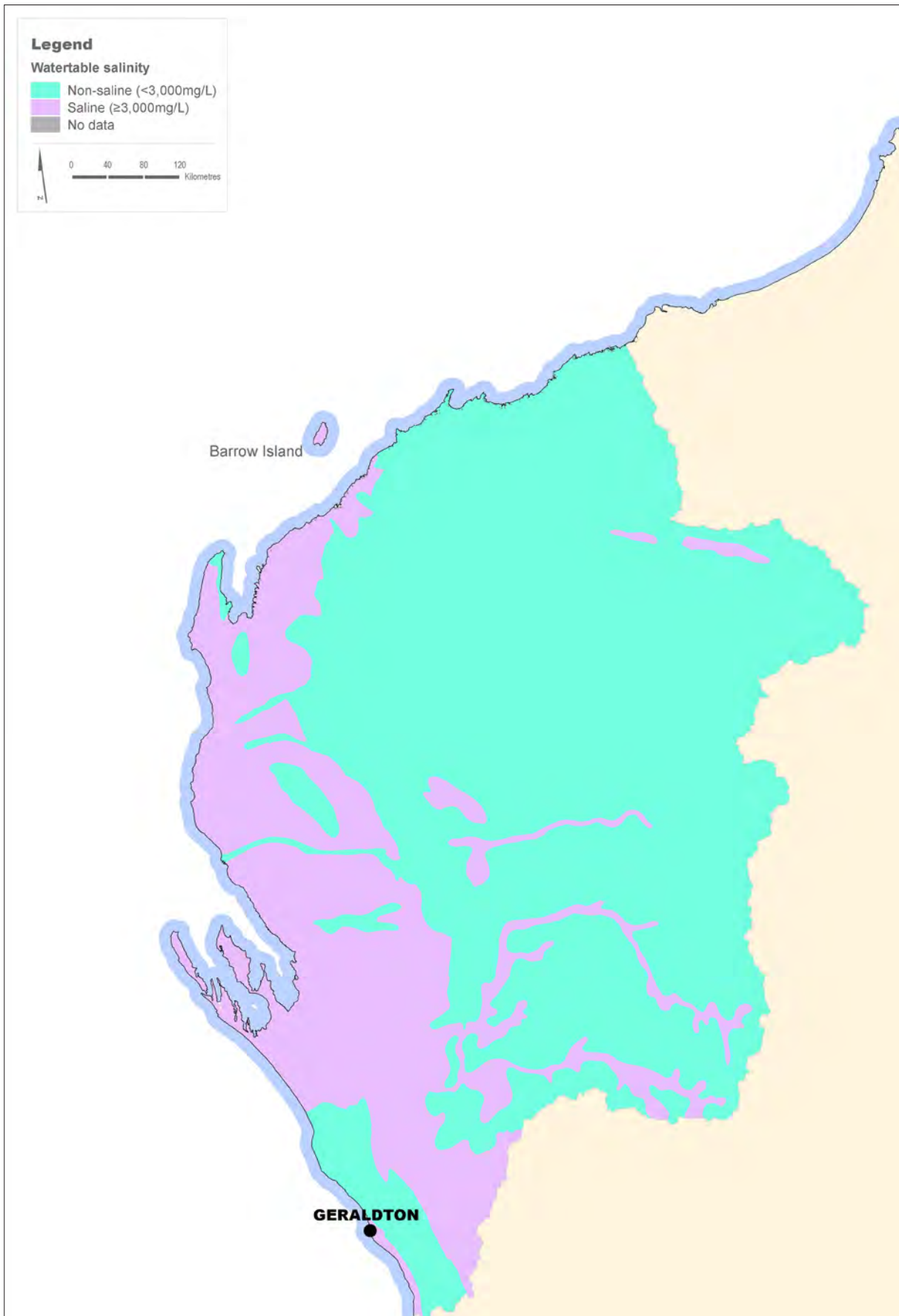
Figure 11.26 Water table salinity classes of the Pilbara–Gascoyne region; data extracted from the Groundwater Cartography of the Australian Hydrological Geospatial Fabric (Bureau of Meteorology 2012)
