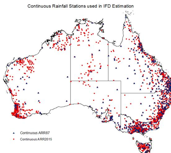
**Figure 3 Comparison of continuous stations used for old IFDs (blue) and those used for new IFDs (red and blue)**
