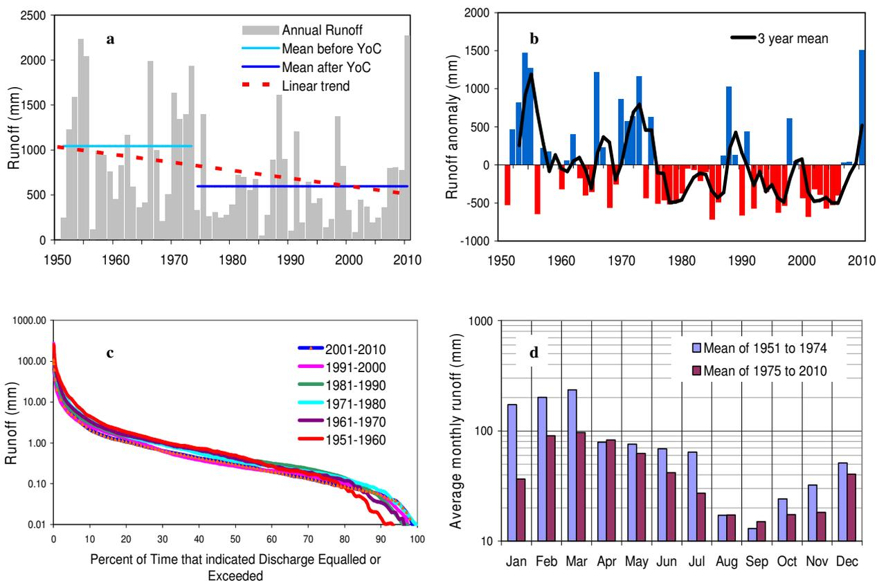
**Figure 3. For Stanley river at Peachester (a) Trend and mean annual flow before and after YoC (b) 3-year moving average (c) Flow duration curves for 6 decades and (d) Mean monthly flow before and after YoC.**
