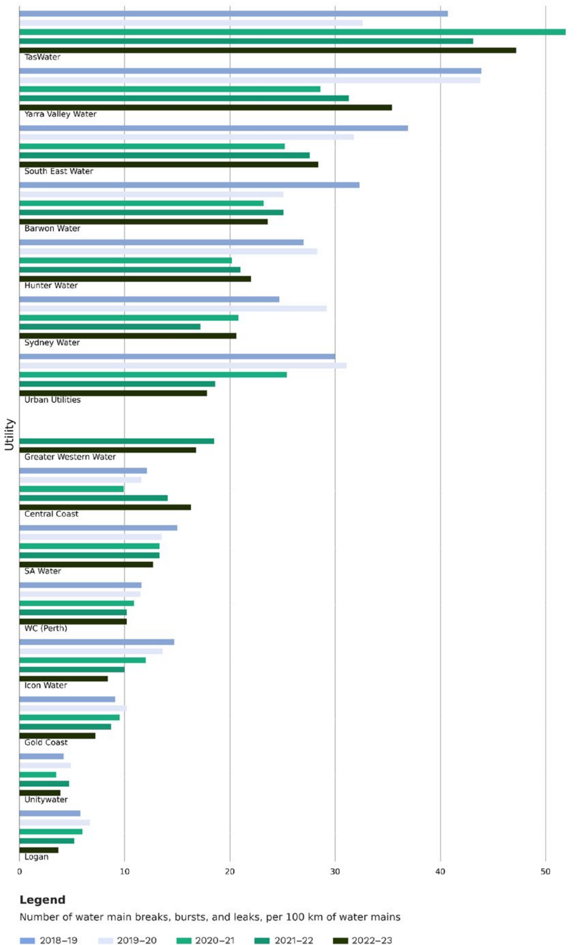
Figure 7.2 Water main breaks, bursts and leaks per 100 km of water mains – Major utility group
