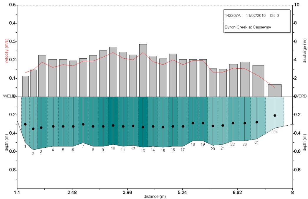
**Figure 4. Example of a good quality gauging – there is a fairly uniform velocity distribution, regular bed and bank shape, and most subsection discharges are less than 5%**
