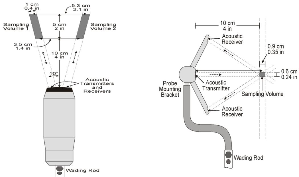
**Figure 1. An illustration of the ADC (left), and ADV (right) point velocity meters**
