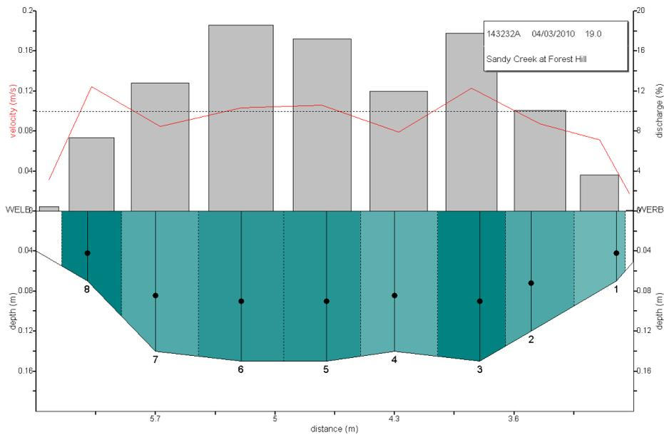
**Figure 2. Example of a poor quality PVM gauging. The measurement contains very few verticals resulting in most intervals containing >10% discharge**
