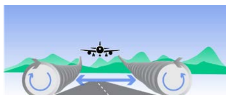
Wake vortices (a) Calm winds: vortices roll apart
