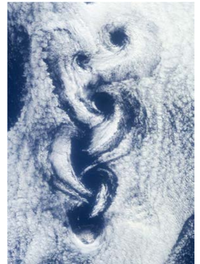
Von Karman vortices forming in a stratocumulus field downwind from the volcanic island of Rishiri-to in the northern Sea of Japan. Credit: NASA
