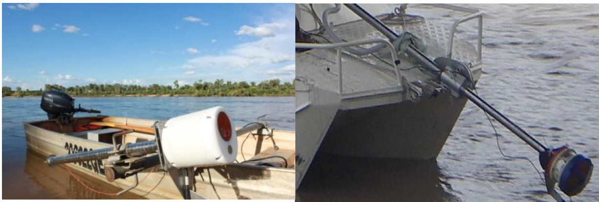
Figure 3. Examples of side (left) and bow mount (right) for a boat.
