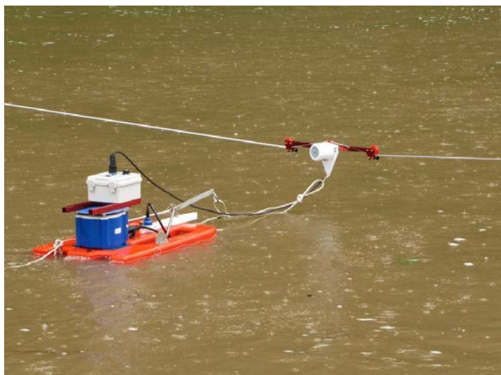
Figure 4. Example of a tethered ADCP deployment utilising a remotely controlled traveller system which ensures a consistent boat speed across the transect
