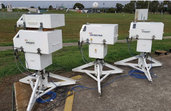
Calibration of Brewer spectrophotometers at the Bureau of Meteorology Training Centre in Broadmeadows, Victoria prior to deployment using the reference instrument from International Ozone Services in Canada (the small instrument on top of the Brewer on the left).
