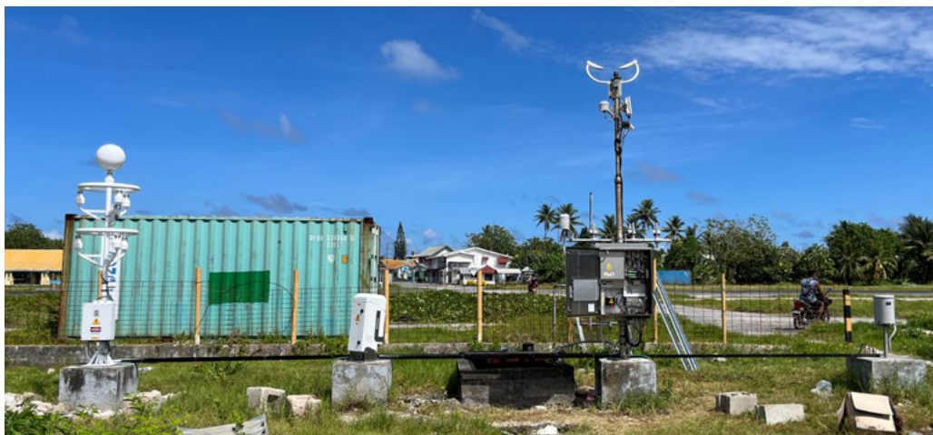
Tuvalu's new aviation weather station located at Funafuti Aerodrome which includes (from left to right) the thunderstorm sensor, cloud sensor, present weather sensor and rain gauge.
