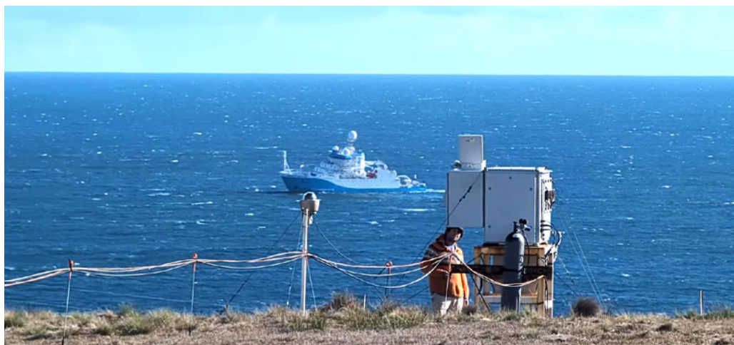
Atmospheric Radiation Measurement (ARM) Technician Tom Day maintaining the Marine Atmospheric Emitted Radiance Interferometer (MAERI) as part of CAPE-k with the RV Investigator around 2 nautical miles offshore. The MAERI is a passive instrument which measures sea surface temperature and other radiative parameters at an above the sea surface. Image credit: Frank Zurek.
